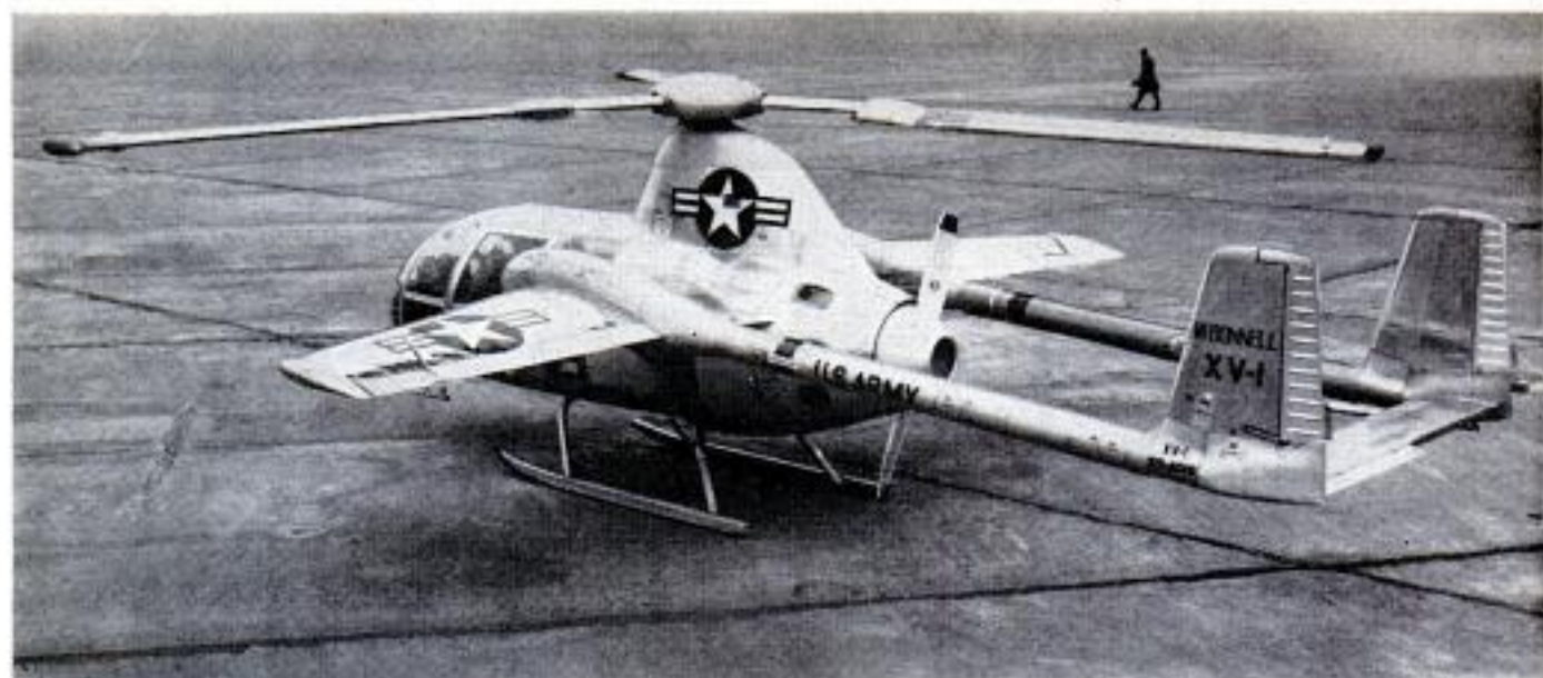
First U.S. military convertiplane is the XV-1, built by McDonnell. Pusher prop and rotor-tip jets power it
